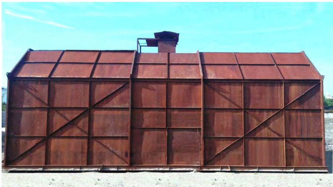
HOUSE FURNACE WITH GAS BURNER FIRING (PWHT) 4m x 4m x 10
